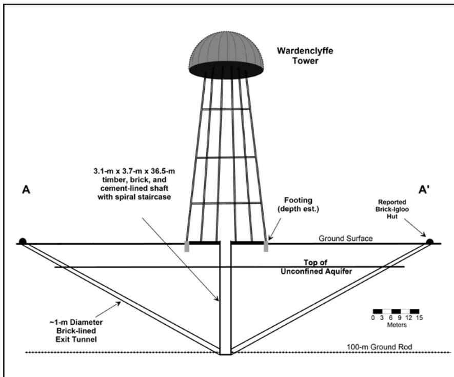
Figure 10. Cross section A–A' showing interpreted location of exit tunnels and vertical shaft beneath the Wardenclyffe Tower.
