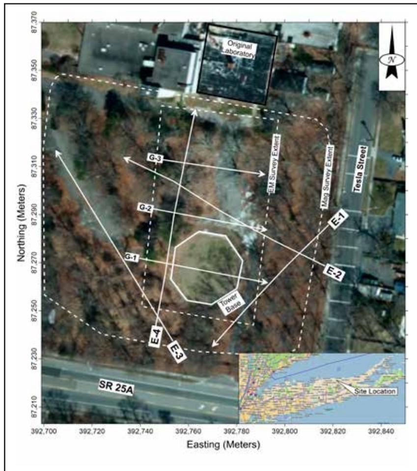
Figure 5. Wardencllyffe plan map showing data collection areas and profile locations. Arrows point in direction of profile data collection. Base map from USGS Earth Explorer (2014) set to Long Island State Plane coordinate system in meters with inset of Long Island, NY.
