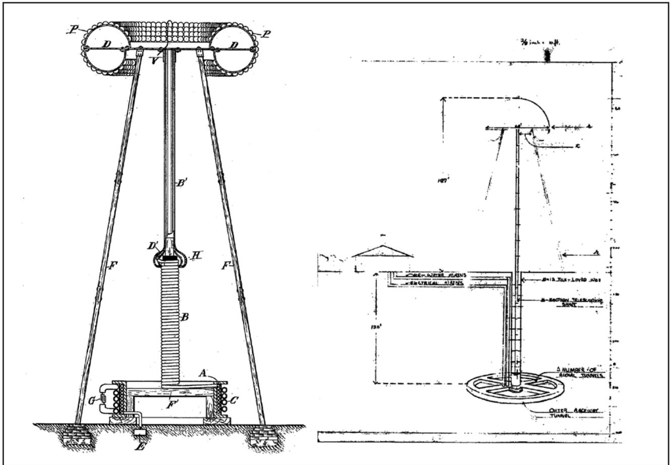
Figure 2. Hand-drawn sketch (right) possibly by Tesla with schematic (left) for Tesla's magnifying transmitter in "Apparatus for transmitting electrical energy." US Patent 1,119,732, filed January 18, 1902.
