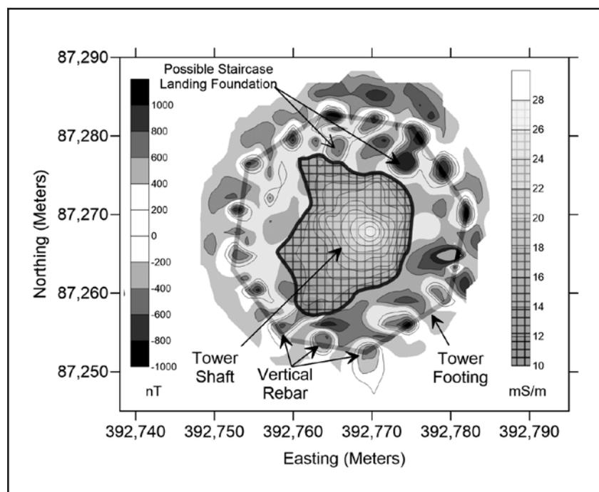
Figure 6. Plan map showing the magnetic susceptibility (nT in solid grayscale) and bulk terrain conductivity (mS/m in crosshatched grayscale) of the octagonal foundation to the Wardencliffe Tower foundation.
