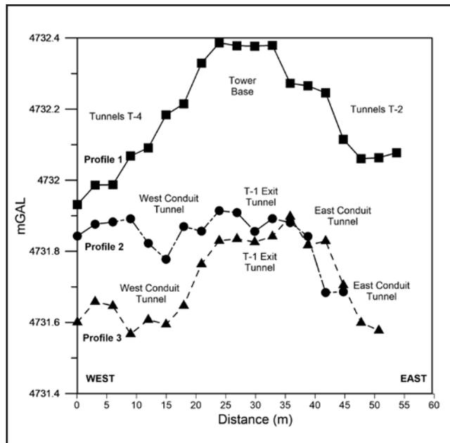
Figure 7. Microgravity profiles showing lower density portions of each profile that are interpreted to be the location of tunnels.
