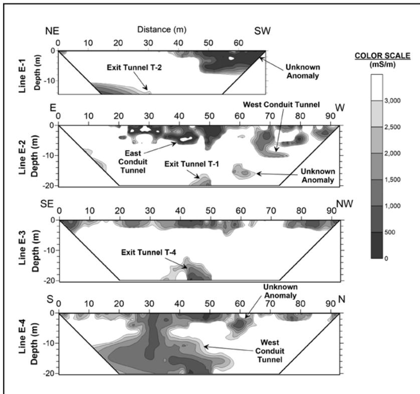
Figure 8. Electrical imaging tomographs showing low conductivity zones interpreted to be brick-lined tunnels. No vertical exaggeration.
