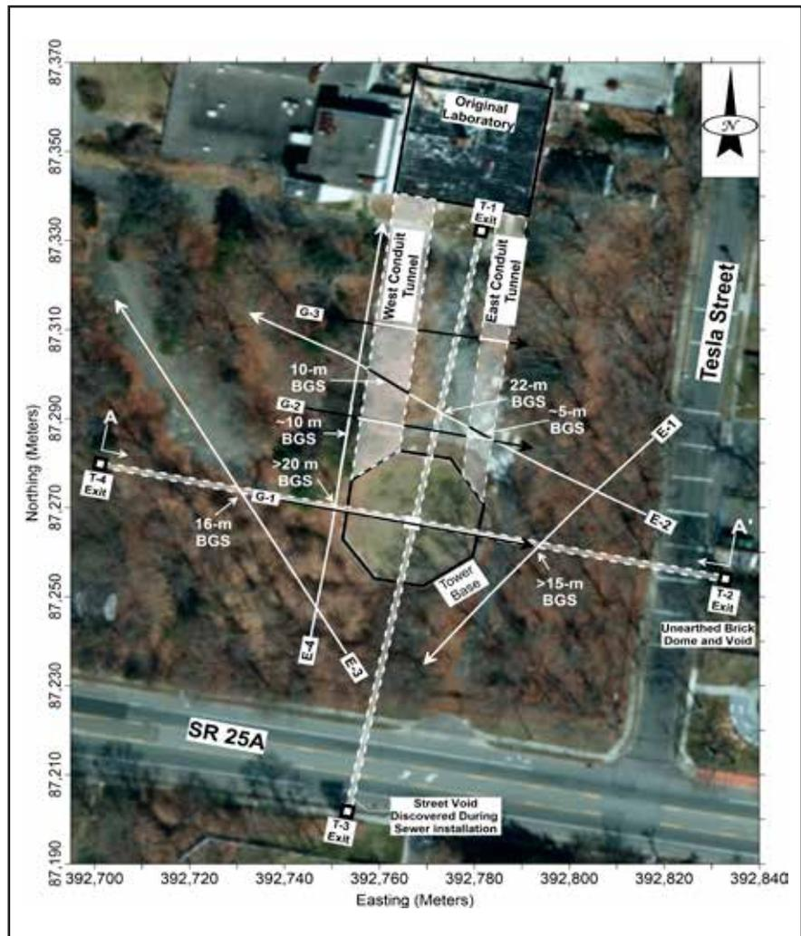
Figure 9. Map of interpreted tunnel locations (dashed white outline) as determined through EI (white) and microgravity (black) mapping with depths shown where detected. West-east profile A–A’ located through the tower base (see fig. 10). Base map from USGS Earth Explorer (see fig. 5).
