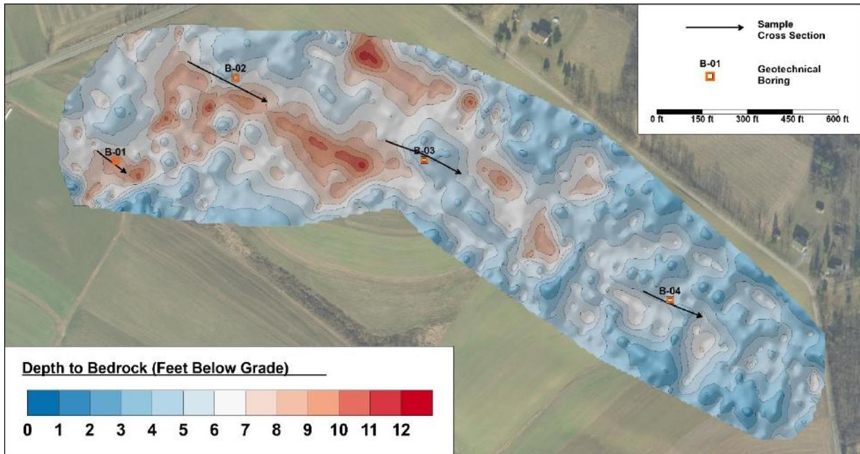
**Figure 4.** Depth to bedrock map derived from TCM data. GIS integration allows for depth to be displayed in units of feet below grade or elevation above mean sea level.
