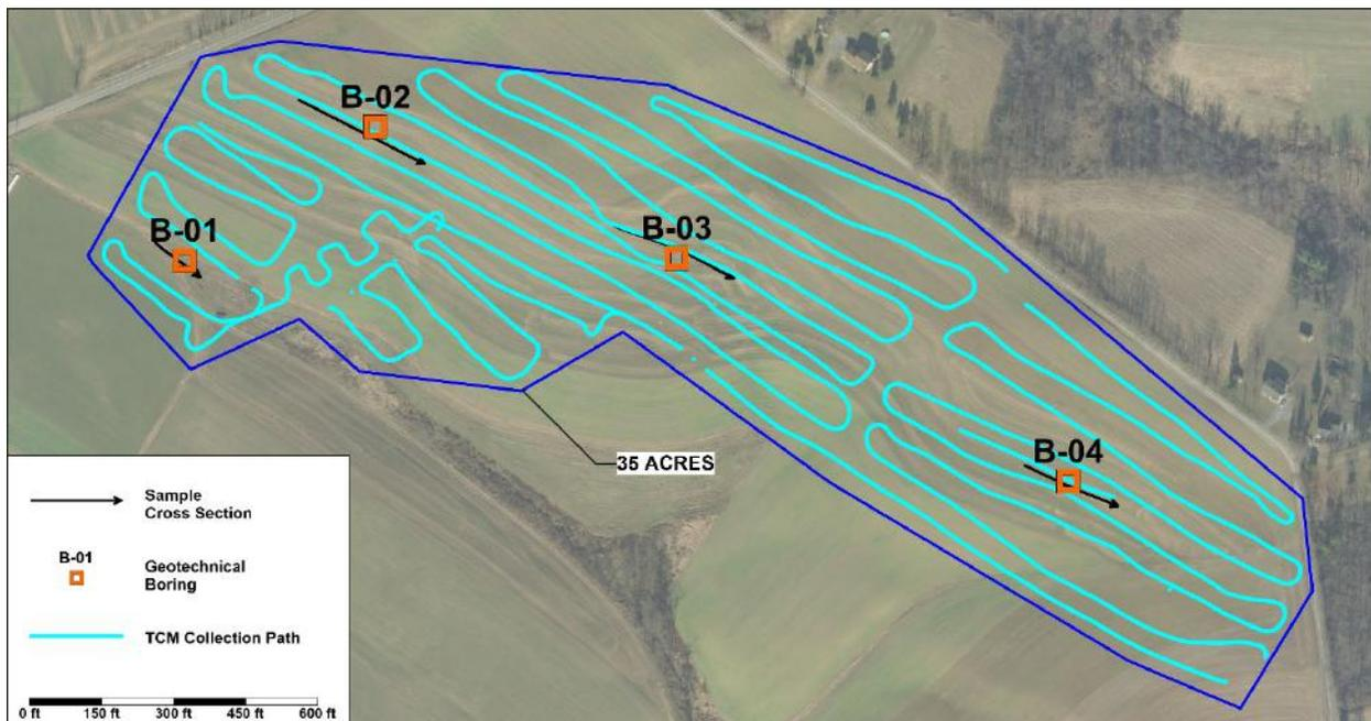
**Figure 2.** Map of UTV-mounted TCM collection paths. Cyan lines represent collection paths with the GF Instruments CMD Explorer instrument. Orange squares are geotechnical borings. Once processed and inverted, cross sections (black lines) were generated over borings to compare resistivity data against known boring data.
