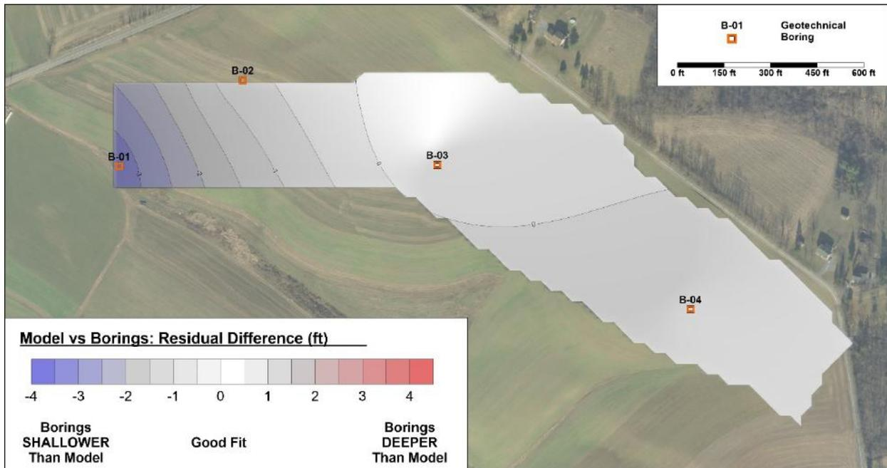
**Figure 5.** Residual difference between modeled depth to bedrock and known depth to bedrock from geotechnical boring data.
