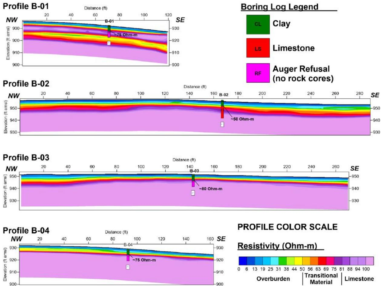
**Figure 3.** Cross section of inverted resistivity data derived from TCM measurements. Existing boring data are overlaid onto the profiles.
