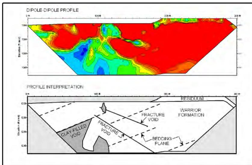
Figure 3. Interpretation of the dipole-dipole CVES profile.
