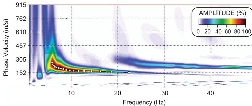
Figure 1. An example of a MASW dispersion curve from south-central Puerto Rico of the fundamental mode of the frequency (Hz) versus phase velocity (m/s). Amplitude intensity is shown in color. The dotted white line represents the fundamental mode. Processed using KGS SurfSeis 3.06 computer program (KGS, 2010).
