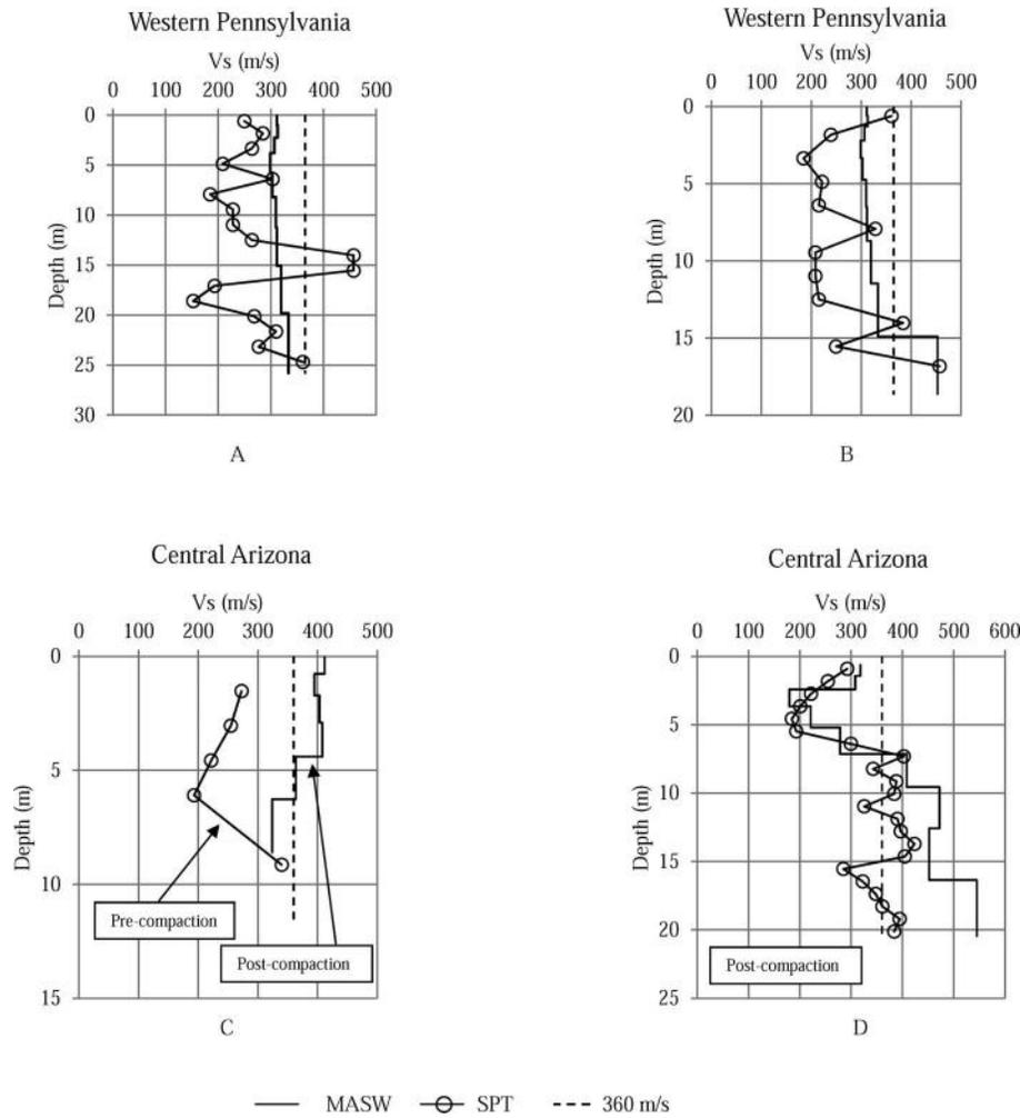
Figure 3. Velocity versus depth profiles for coal mine spoil from western Pennsylvania and C&D waste from central Arizona. Diagram C shows pre-compaction SPT-derived  $V_s$  with post-compaction MASW-derived  $V_s$ . Diagram D shows post-compaction SPT- and MASW-derived  $V_s$ .
