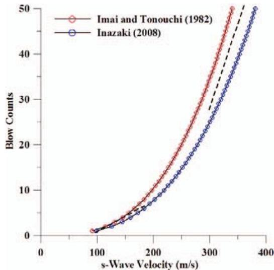
Figure 2. Continuous blow counts converted to  $V_s$  using regression equations from Imai and Tonouchi (1982) and Inazaki (2006). Note dashed straight line functions from  $N$ -value of one to six blows and from 30 to 50 blows.
