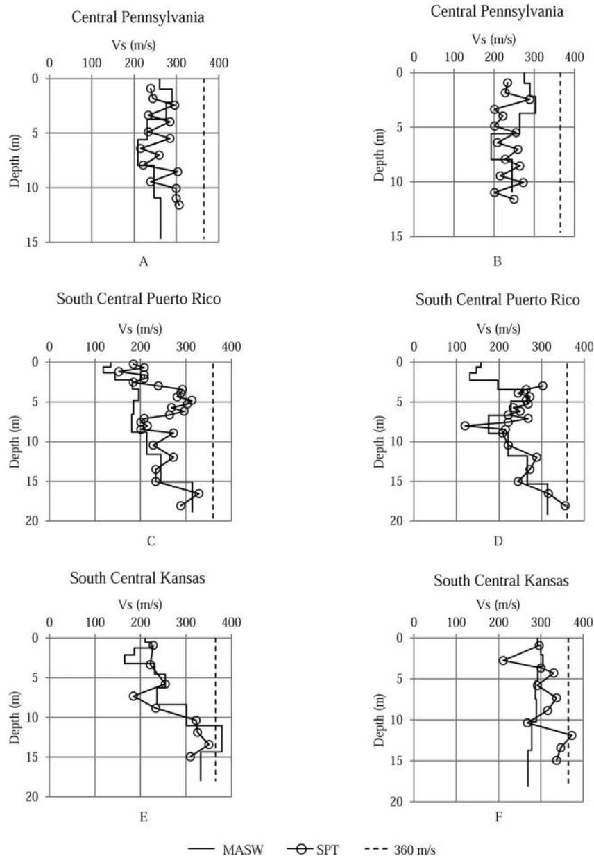
Figure 5. Velocity versus depth profiles of fluvial deposits from central Pennsylvania, south-central Puerto Rico, and south-central Kansas.
