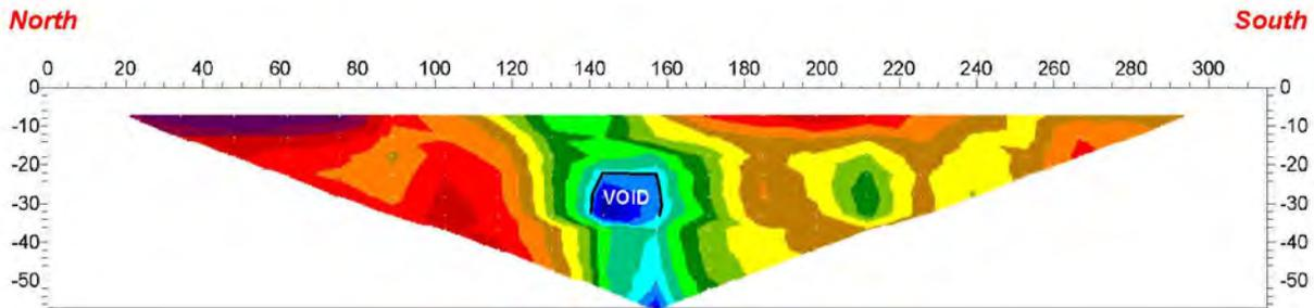
Figure 11 Electrical imaging profile of a karst void (no vertical exaggeration, in feet)
