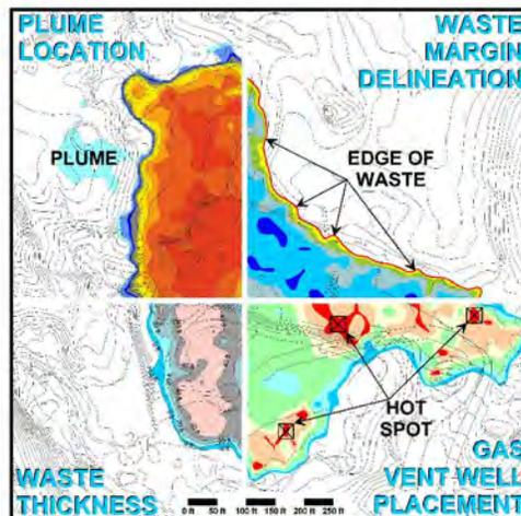
Figure 5 Processed FDEM terrain conductivity data, showing waste margin, inferred depth of waste, waste thickness and areas of gas-generating bacterial activity using various processing algorithms (units as shown or relative).
