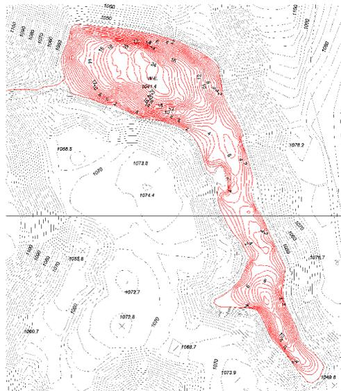
Figure 8 Depth of water (in red) in an abandoned surface-mine lake in Ohio (scale, 1 cm equals 50 meters; contour interval 2 feet).
