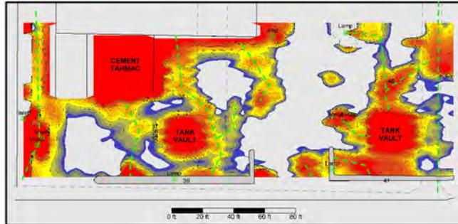
Figure 4 TDEM map of underground storage tank locations (blue to red are low to high millivolts, respectively).
