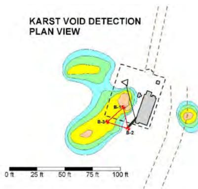
Figure 12 Plan map of karst voids showing depth to top of voids (color scheme; 10 meters [tan] to 25 meters [blue] below grade in 5-meter increments).
