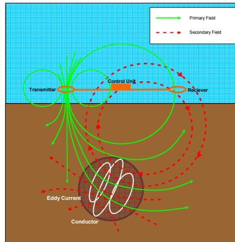
**Figure 1:** A diagram of the transmitter-receiver orientation of the EM tool. The transmitter creates the primary electromagnetic field that generates eddy currents within the conductor that are measured by the receiver (McNeill, 1990).
