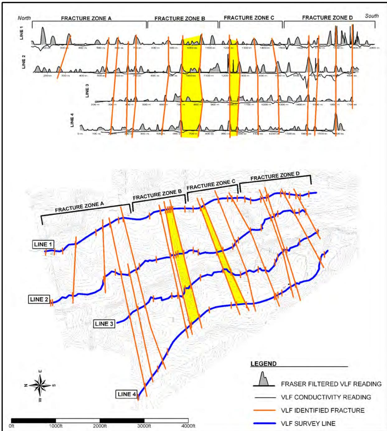
**Figure 3** Fraser-filtered VLF survey lines showing fractures (above x-axis) and fluid conductivity (below x-axis) and interpretation of the fracture pattern on the topographic map.
