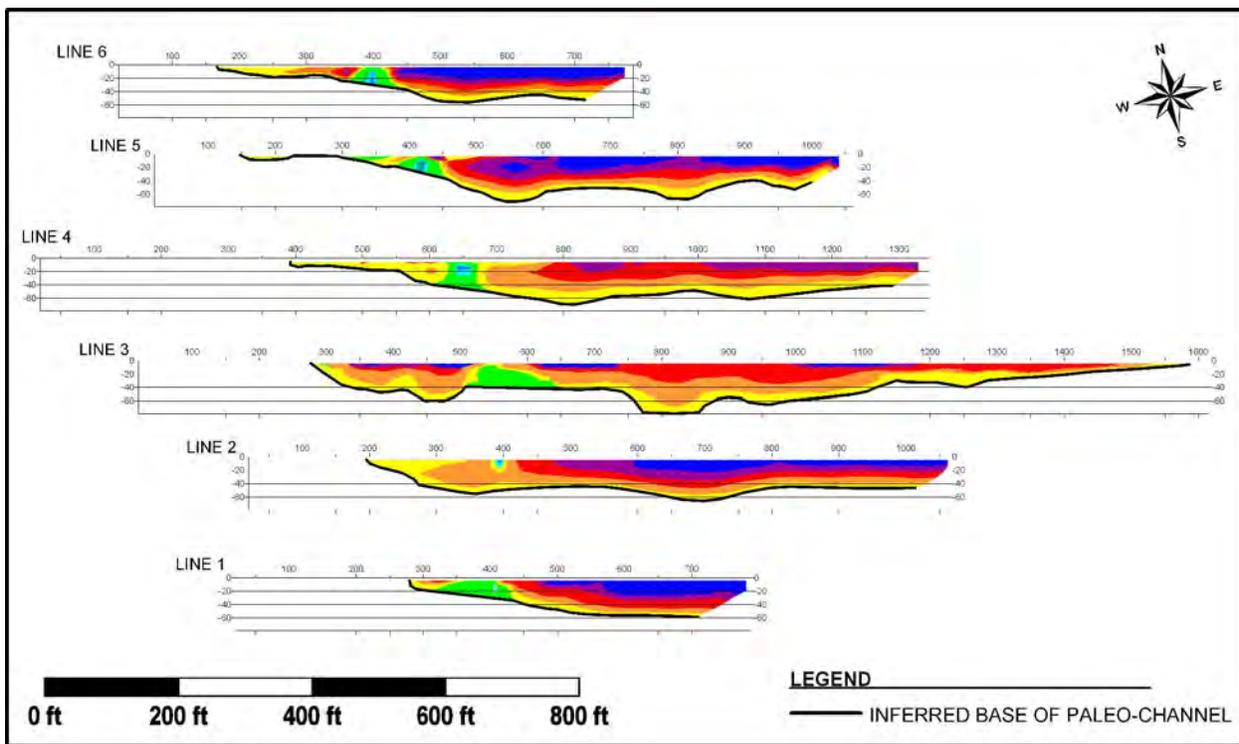
Case 1 study consisted of defining the horizontal and vertical extent of the paleo-channel for placement of production wells using resistivity. The unconsolidated channel sediments are estimated to have resistivity values of less than 40 Ohm-meters; whereas, bedrock (i.e., Paleozoic shale and sandstone) is estimated at greater than 40 Ohm-meters.
