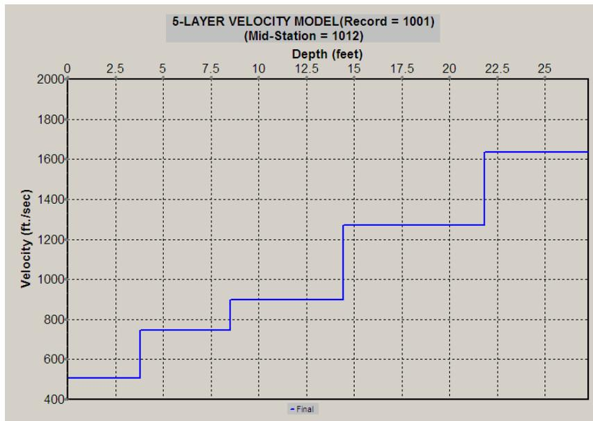
**Figure 6:** Velocity profile derived from the inversion of the MASW fundamental-mode dispersion curve using a simple 6-layer model.
