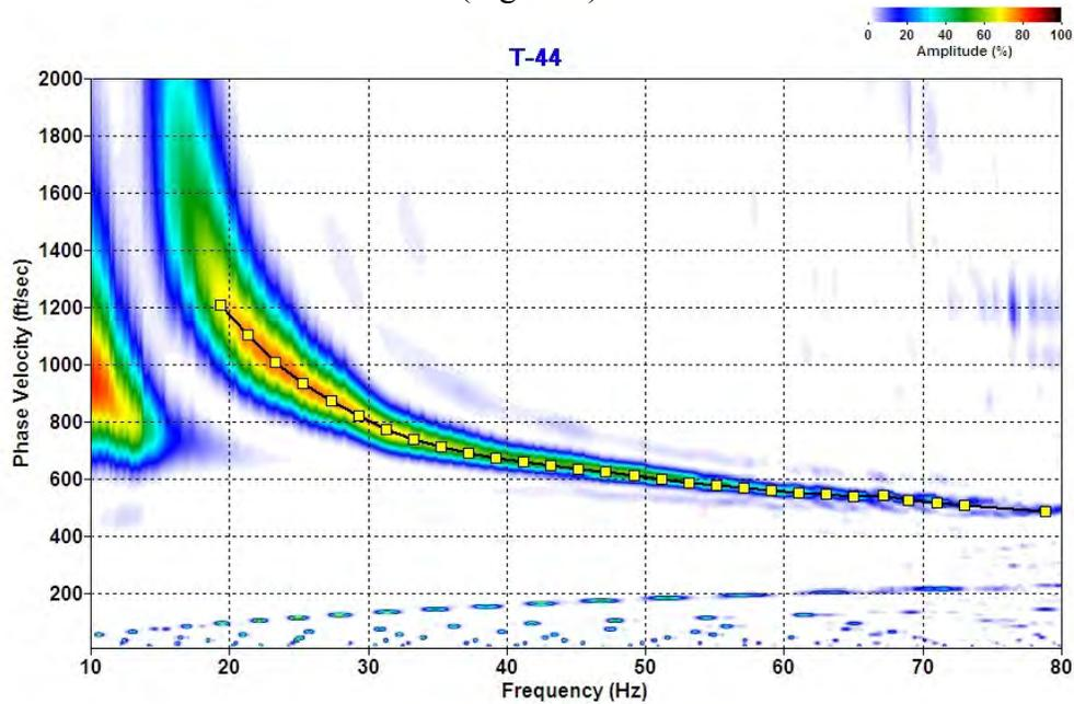
**Figure 5:** The fundamental-mode dispersion curve has been extracted from the dispersion overtone graph for this soil site in Wyoming. An inversion of the fundamental-mode dispersion curve produces a reasonable velocity profile that nearly matches the VSP-derived shear-velocity profile.
