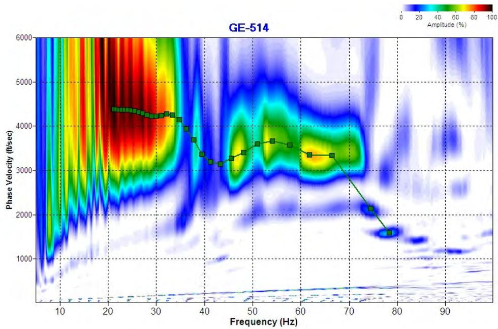
**Figure 3:** Dispersion pattern (phase velocity vs frequency) for a bedrock setting (i.e., rock at the surface); note the fundamental-dispersion curve is poorly developed and little useful data is present for the interpretation of the shallow portion of the rock record (i.e., higher frequencies).
