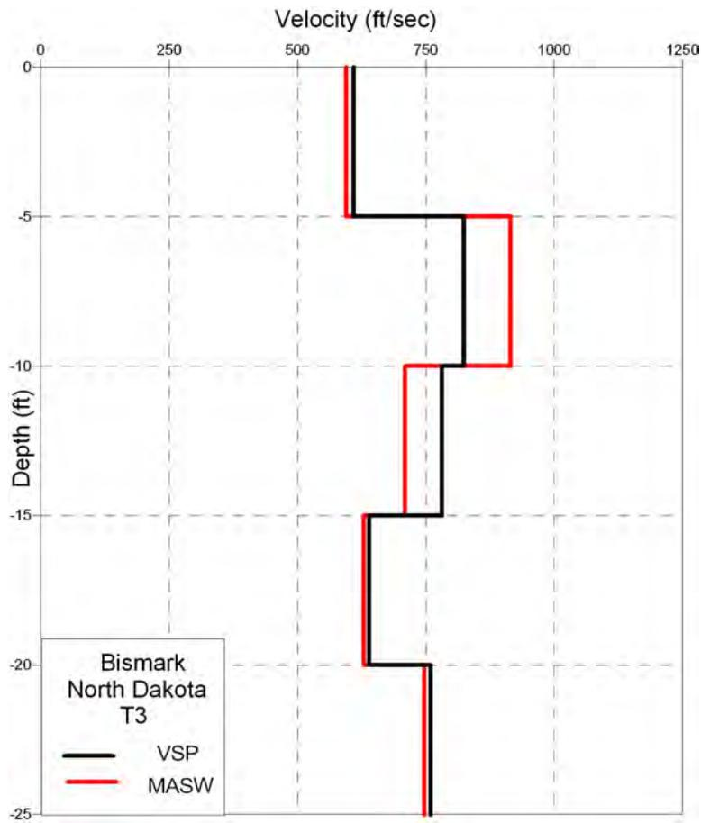
**Figure 2:** Shear-wave velocity-versus-depth curve for a glacial till showing VSP- and MASW-derived profiles.
