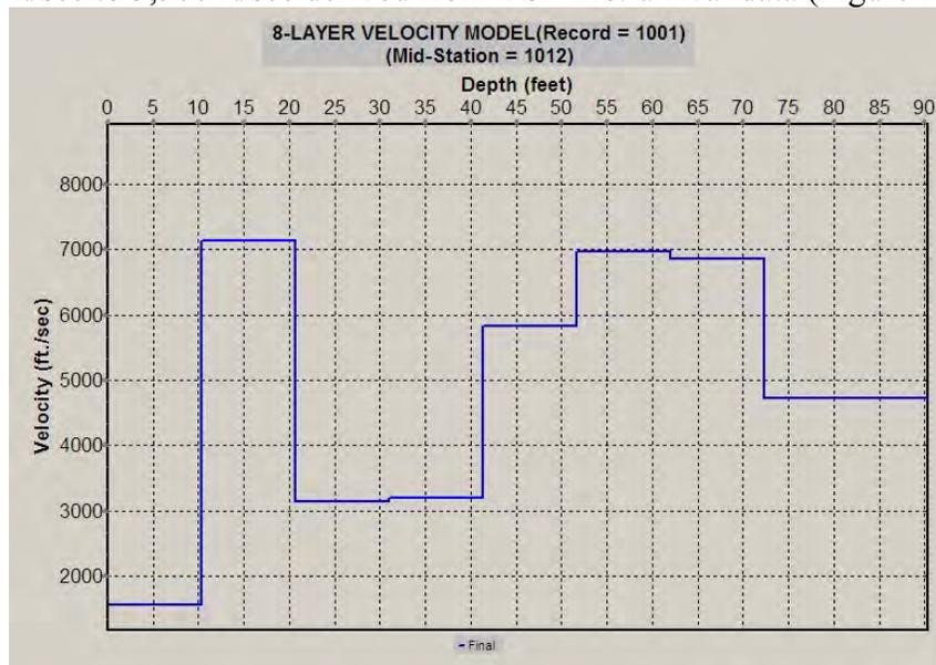
**Figure 4:** Shear-wave velocity profile generated through MASW methods for a rock site in Texas; note that interval velocities are well above those considered reasonable for this area and generated through VSP methods (i.e., derived from the first-arrival data).
