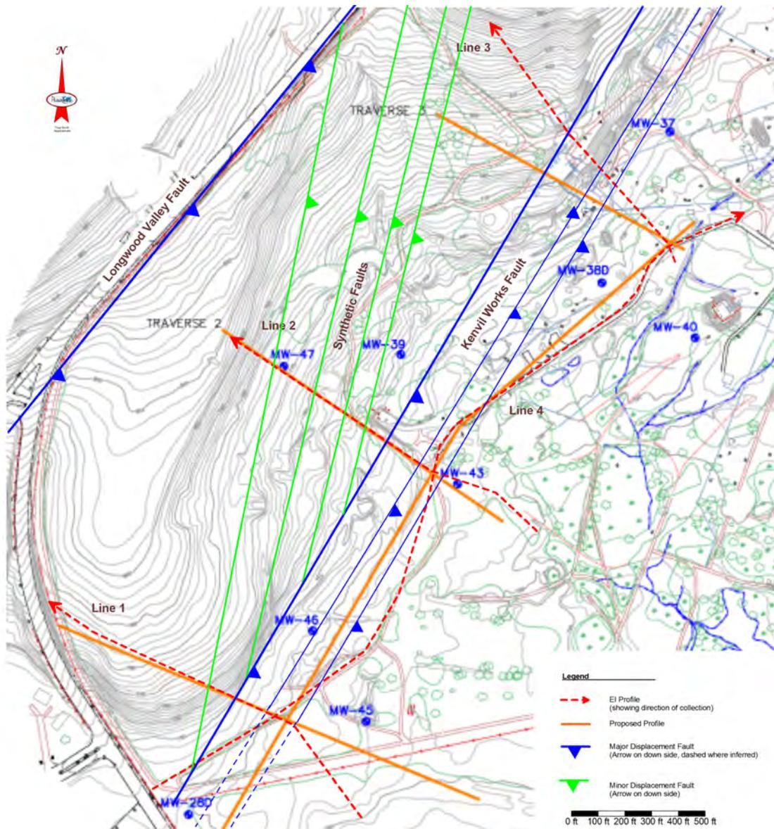
**Figure 3:** Topographic map (contour interval 2 feet) showing geophysically-derived interpreted faults.
