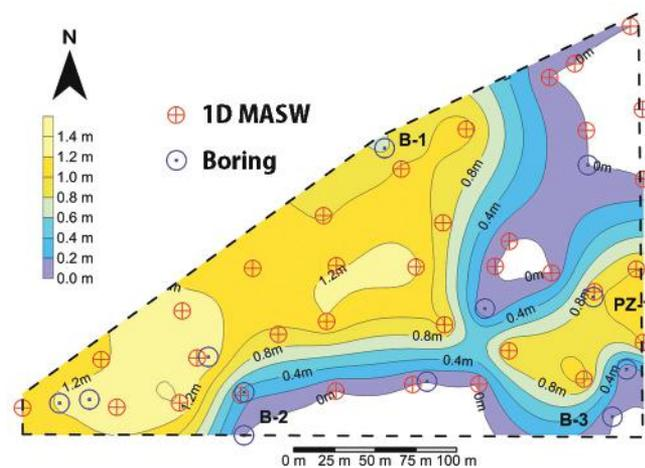
**Figure 4.** A 90,000-square-meter wetland located in upstate New York contiguous to a landfill (not shown) showing MASW test sites and subsequent boring locations. Piezometer PZ-1 was predicted by MASW method to have a 0.7 m thick, lacustrine clay bed, when in fact, this boring had a 0.85 m thick clay layer. Color scale represents thickness of clay in meters.
