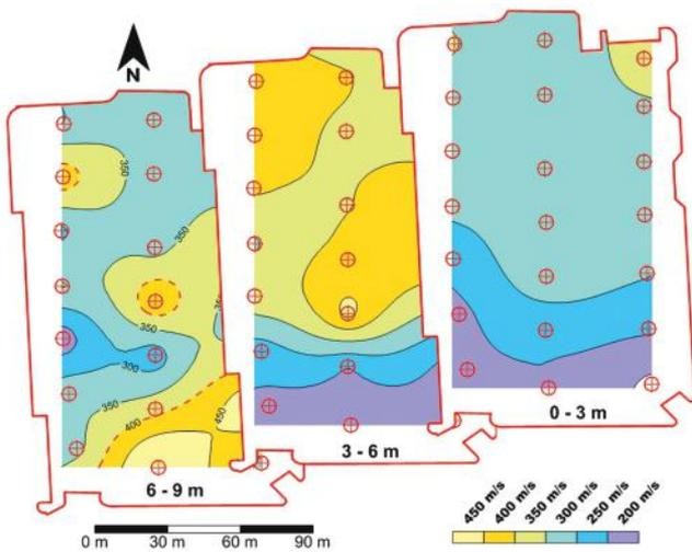
**Figure 3.** Three shear-wave interval velocity-at-depth maps of a proposed 16,000-square-meter industrial facility (red solid line is the building footprint) in Arizona showing 1D MASW test locations (red symbol). Interval depth ranges are posted at the bottom of each image. Red dashed line at 6–9 m below grade represents top of rock.
