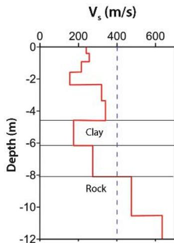
**Figure 1.** MASW derived shear-wave-velocity depth graph (red) from a site in upstate New York. Rock is arbitrarily placed at the shear-wave velocity of 400 m/s (dashed line).
