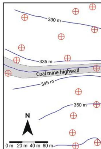
**Figure 2.** Plan map of a portion of the proposed hospital in western Pennsylvania showing the highwall and MASW test locations (red symbols). Several of the MASW test locations are located near borings (not shown) to help truth the shear-wave-velocity data. Blue contour lines represent top of rock in meters above sea level.
