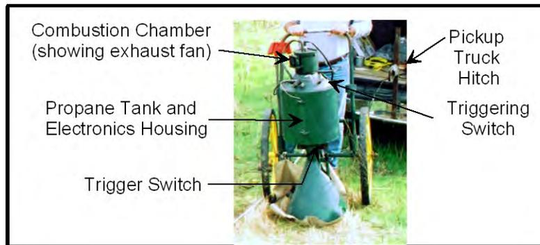
Figure 1: Seismic gun in preparation for a shoot, showing compactness and portability. The triggering switch initiates the filling of the combustion chamber with propane gas and subsequent firing of the gun through an automobile spark plug. The trigger switch adjacent to the vertical sonic or exhaust tube starts data collection. Exhaust fan purges the exhaust gases from the combustion chamber in preparation for the next event.
