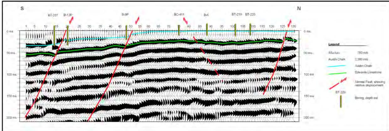
Figure 5: MSF profile collected from south to north along Red River Avenue, showing interpreted faults. Note that the apparent dip is consistent with field measurements of rock strata. Profile was collected on a relatively horizontal road (<2 m elevation change across profile).
