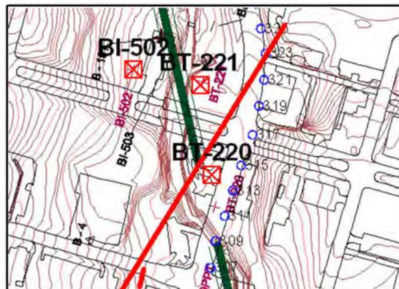
Figure 7: Boring location BT220 in relation to the Waterloo Park Fault (in red, throw is down to the right). Alignment (in green) passes through this fault (base from KBR, 2008). Scale 1 cm = 18 meters; true north to top of page.
