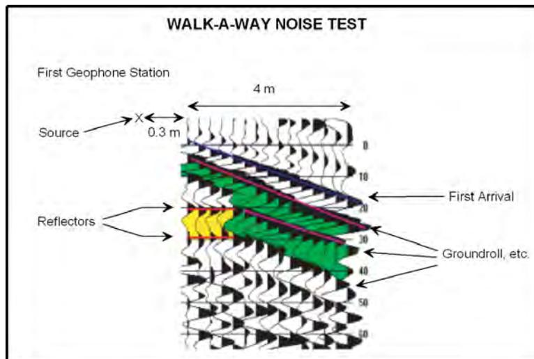
Figure 2: Walk-away test for MSF system where the phase and group velocities are in-phase approximately 1.2 meters from the source. The geophone-source separation must be less than 1.2 meters to assure that the event observed at 20 ms is a reflector and not ground-roll or other type of wave form.
