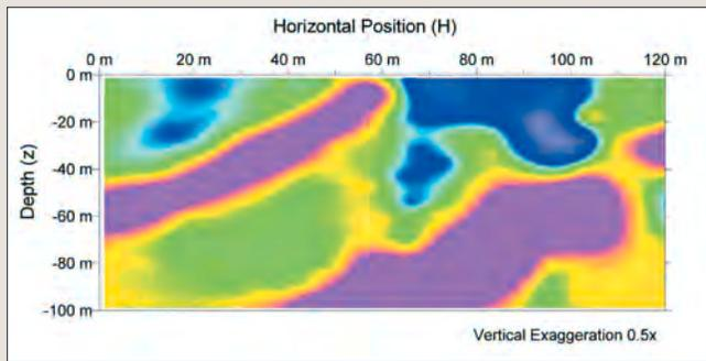
**Figure 3.** Processed depth profile of VLF current density measurements showing statistical projections of fractures at depth. Fracture package located at the edge of a deep longwall panel mine in southwestern Pennsylvania.
