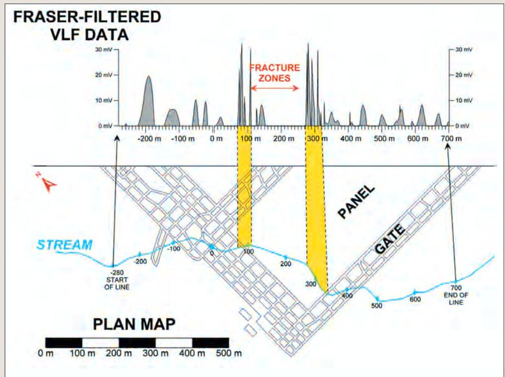
fractures (50-80 m; Figure 5). The fractures appear to dip into the center of the panel due to the tailing off of the tilt-angle reading toward the center of the panel.
