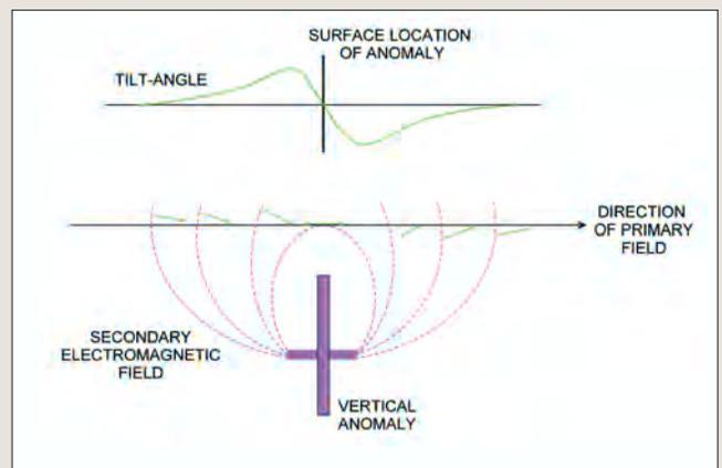
Figure 2. Tilt-angle profile over a vertical anomaly.
